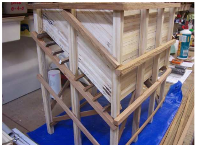
Piers, walers, joists and bracing in place ready to tackle the mechanism that releases the Coal.
