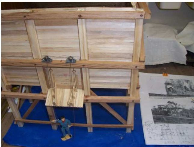
Gate lift mechanism comprises; side guides, plumber blocks, pulleys and chain.
