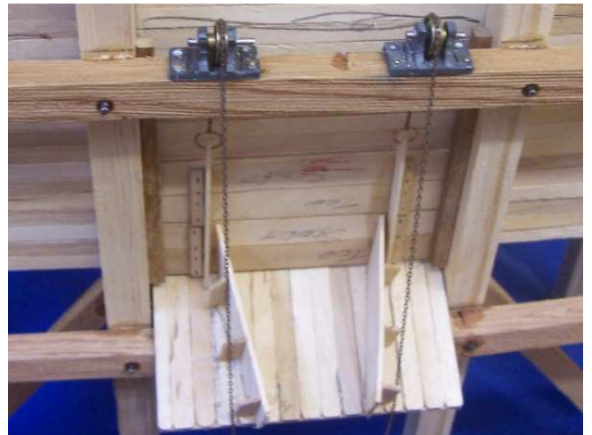
Gate lift mechanism comprises; side guides, plumber blocks, pulleys and chain.
